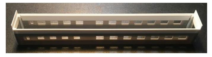
Once the body assembly was square, cemented, and dried, I glued on the roof, making sure to get a tight joint. After it was dry, I filed the ends to fit the roof contour. (Sanding particles still showing on photo of end.)
