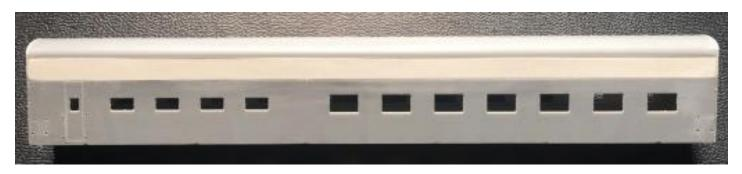
To make sure the extensions were blended into the sides, I filled in the areas with putty and sanded it down. I took my time on this, pausing to reprime and add putty before my second sanding pass. Here we see the side with the first application of putty, and then the finished side after the second filling and sanding pass.
