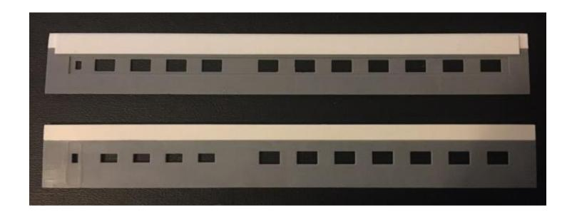
Luckily, I didn't have to change the windows or doors like on Tavern/Lounge #7602. I added two hundred thousandths of an inch (0.200") to the height of the sides. The upper part of the picture above shows the interior of that side. Note the reinforcement strip to strengthen the joint.
