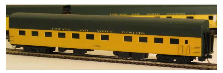
And here's the finished model of Diner number 6954 with American Limited working diaphragms installed and Micro-Trains 4 wheel passenger trucks.
