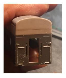
After assembly, the next step was to drill grab iron holes.
